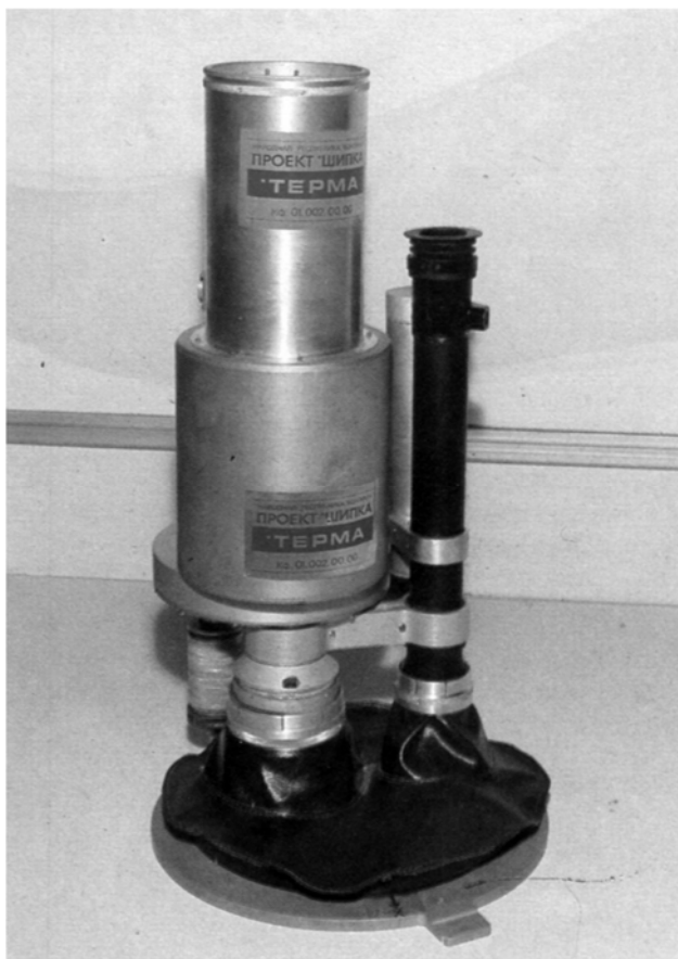
Fig. 10. External view of impulse photometric equipment “Terma”
